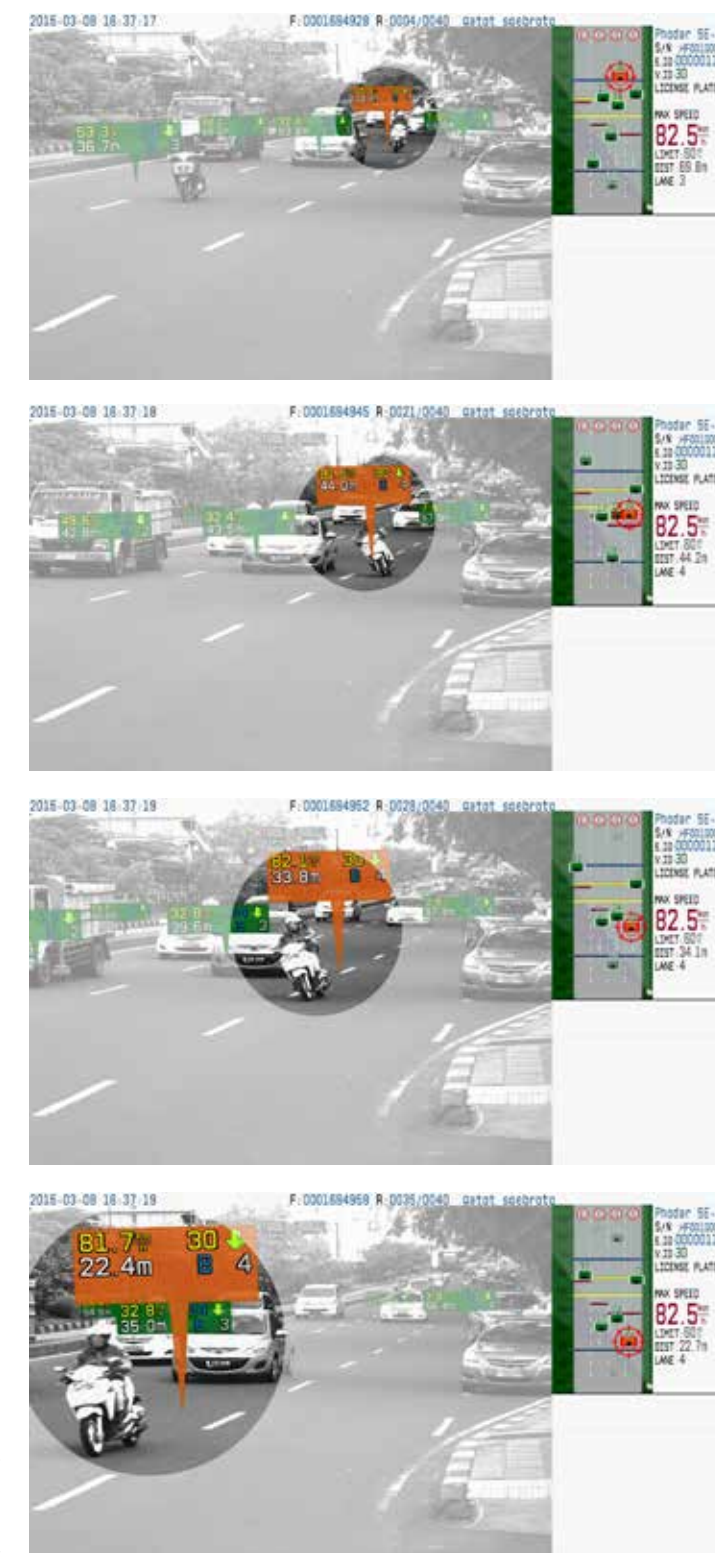
In this sequence, sophisticated tracking algorithms follow a speeding motorcycle changing lanes along a narrow, crowded highway
