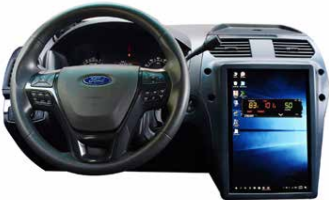
The Havis Integrated Control System (developed by a partnership of Ford, Lectronix, and Havis) in the 2013 and later Ford Interceptor Sedan and SUV
